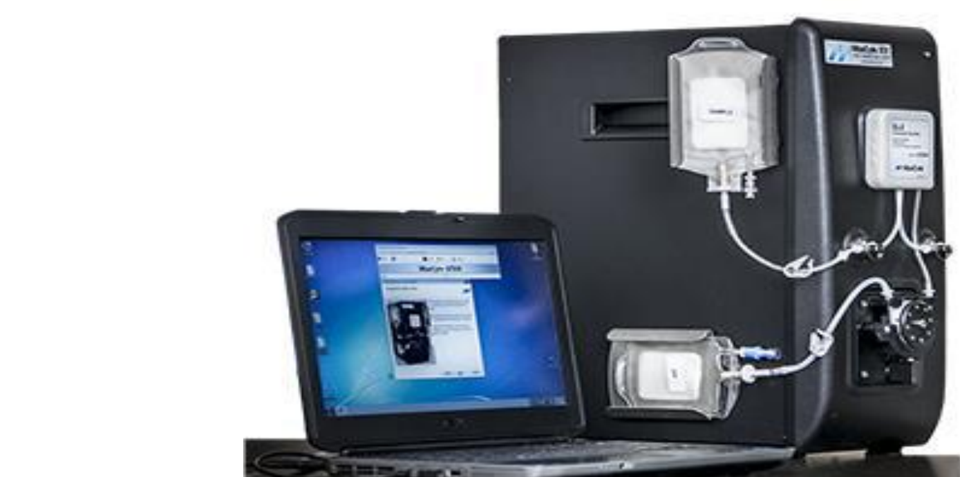
Figure 2. MaxCyte® STX electroporation transfection apparatus. Pictured is the apparatus set up for 100mL flow electroporation and expansion to a 4L culture. The experiments described here utilized the 0.4mL cuvette and 15mL culture volumes.
